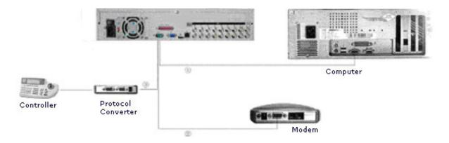
Note: The connection for DVR system software upgrading or debugging through the serial port The connection for dial-up login through MODEM The connection for DVR control through keyboard
